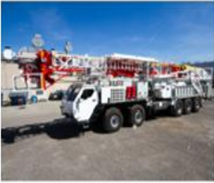
Mobile heavy duty Double Workover Rig 90 tons
